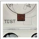
Simulate "trip"(make NO, NC contacts act) to check the control circuit
