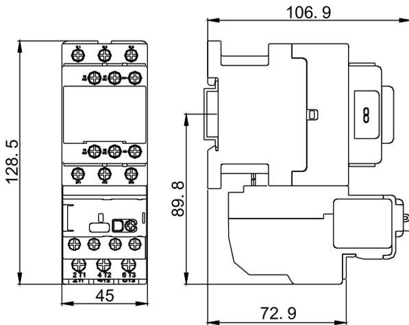
HDRX-38 With HDCX-25/32/38 DC Assembly Installation
