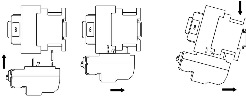
Installation method 1: Install the contactor to the DIN rail, then install the thermal relay
