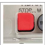
Make the NC contacts act, but not affect the NO contacts. When push STOP button, the control circuit will be open, and motor stops working.
