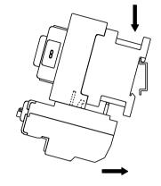
Installation method 1: Install the contactor to the DIN rail, then install the thermal relay
