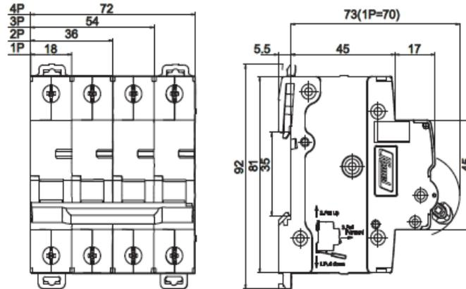
Fig. 3 Overall dimensions of installation
